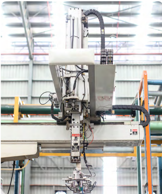
Automated handling systems at Toyoplas’ plastic injection moulding machines.
