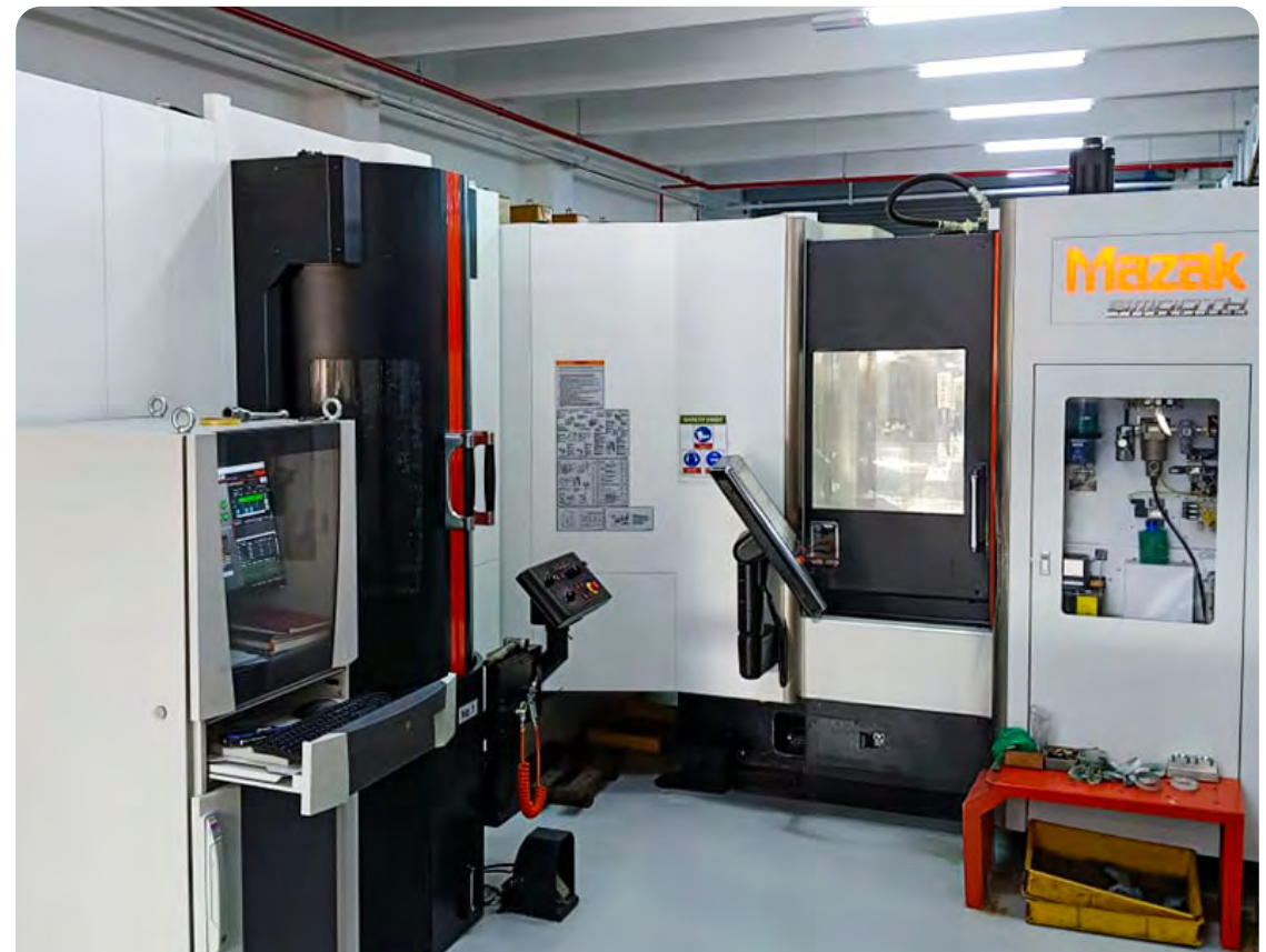
A modular, high-efficiency system designed to automate pallet handling and workpiece management for CNC machining.
