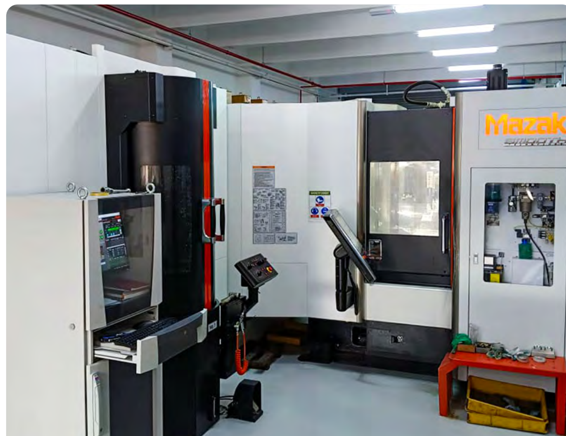
A modular, high-efficiency system designed to automate pallet handling and workpiece management for CNC machining.
